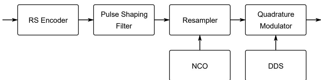
**Figure 1. The RS-QPSK Modulator IP Core block diagram**
