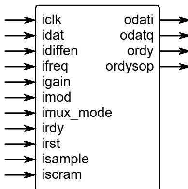
**Figure 3. The RS-QPSK Modulator port map****Table 1. The RS-QPSK Modulator port map description**
