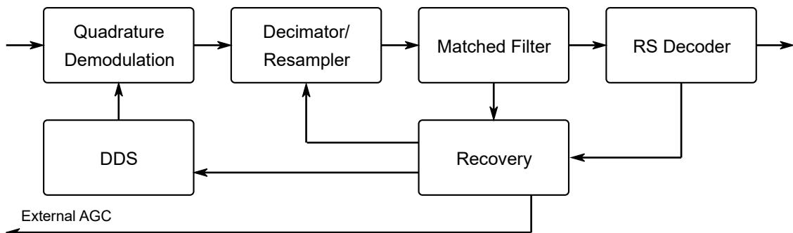
**Figure 2. The RS-QPSK Demodulator IP Core block diagram**
