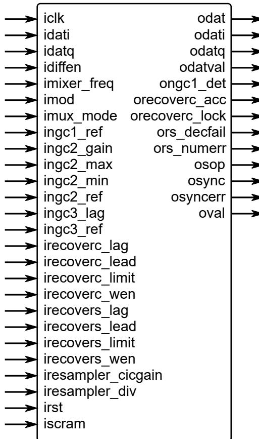
**Figure 4. The RS-QPSK Demodulator port map****Table 2. The RS-QPSK Demodulator port map description**
