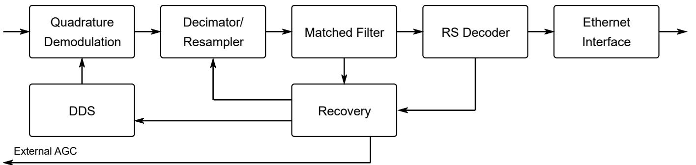
**Figure 2. The Multi-gigabit Demodulator IP Core block diagram**
