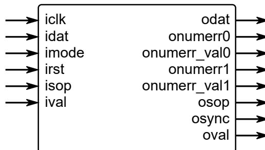
**Figure 4. The I.9 BCH Decoder port map**
