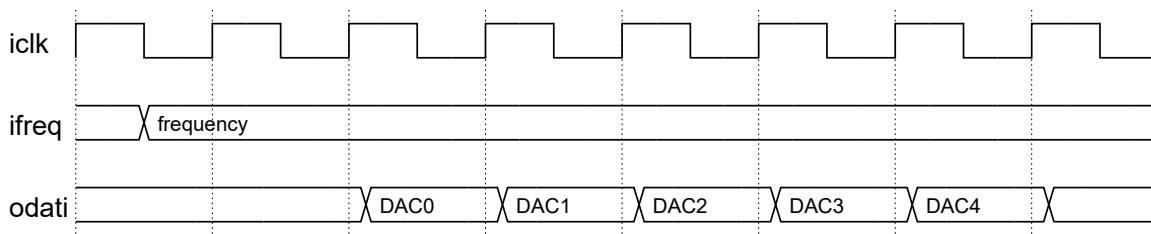
**Figure 6. The timing diagram for IF mode.**
