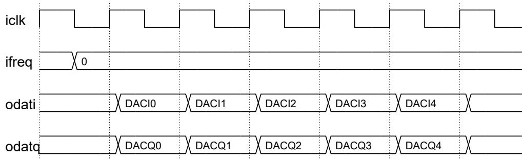
**Figure 4. The timing diagram for baseband mode.**
