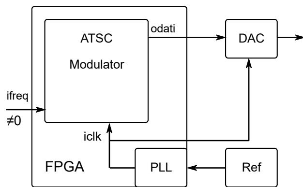
**Figure 5. The DAC connection diagram for IF mode.**
