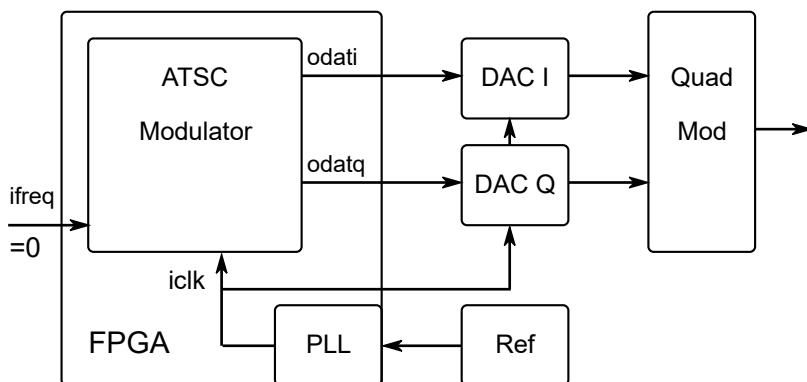
Figure 3. The DAC connection diagram for baseband mode.
